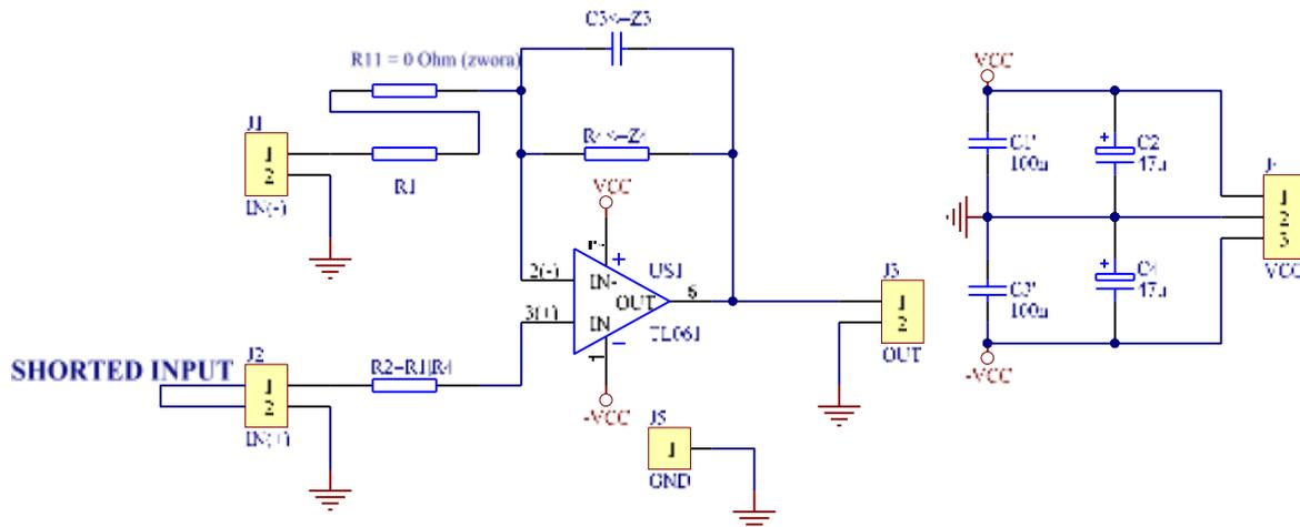
Fig. 2 Inverting amp schematic diagram.
