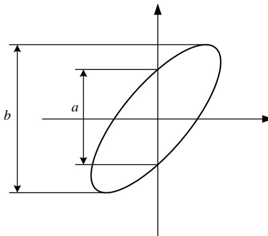
Fig.A.2. Idea phase shift measurement in XY regime of the scope
