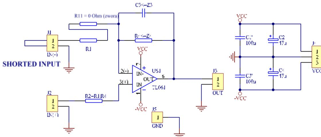
Fig.3., Non-inverting amp.
