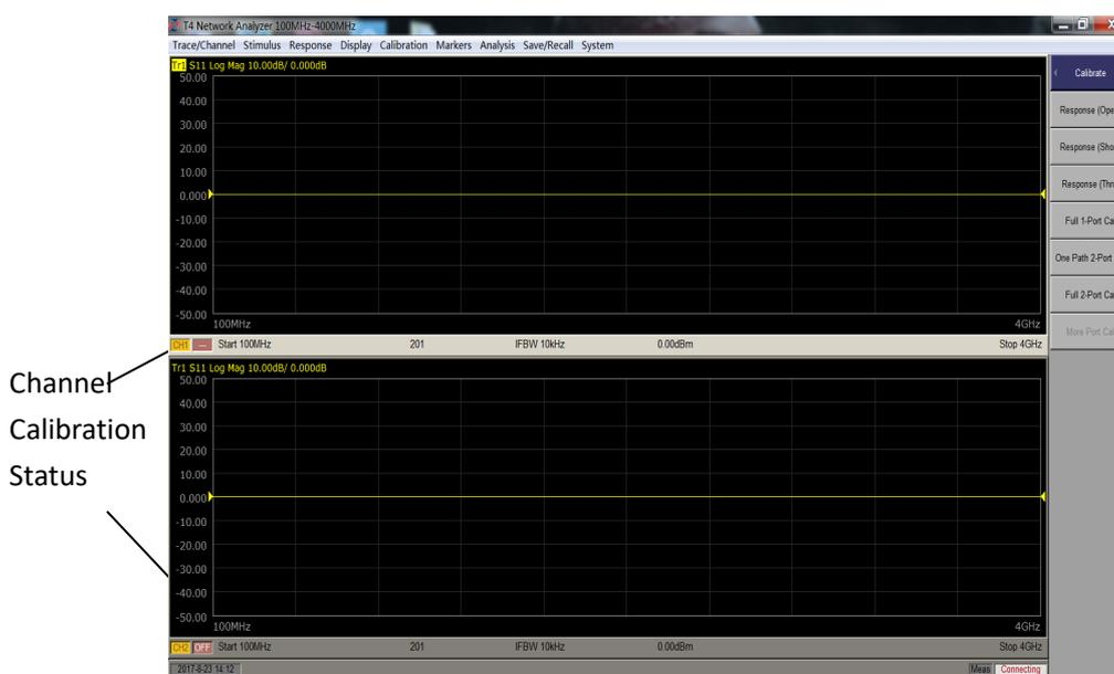
Figure 3-1 Channel calibration status
