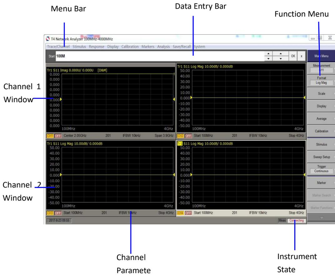
Figure 1-7 Instrument Display Interface
