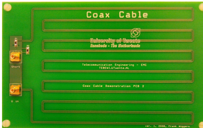
Figure 3.1: The Finished Coax Cable Board.
